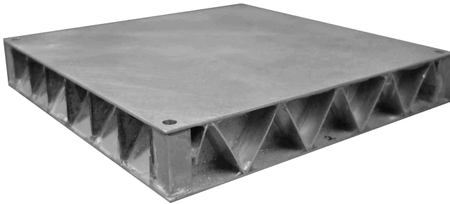
Fig. 9 Vertical bicell and horizontal triangular corrugation test panel.
